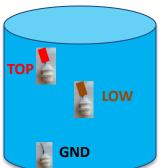
**COLOUR CODE:** for connecting wires
