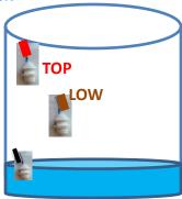
STATUS: when the water in the tank once reaches the top level, the motor will stop. The top and bottom level will start glowing OHT TOP: yellow led GLOW
